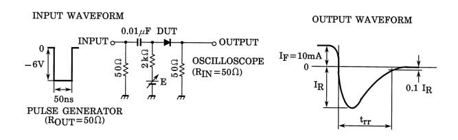
Fig.1 Reverse Recovery Time (t<sub>rr</sub>) Test Circuit
